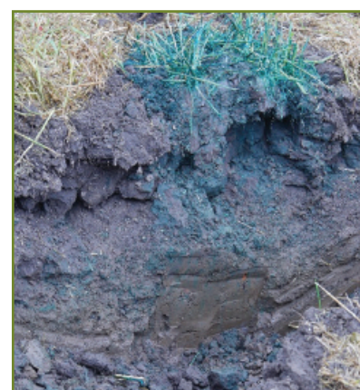
Ink infiltration tests have shown the impact of roots on water infiltration.
