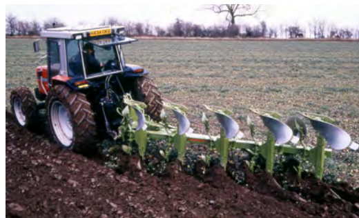
Good ploughing is dependent on correct set-up, effective use of skimmers and favourable soil conditions.
