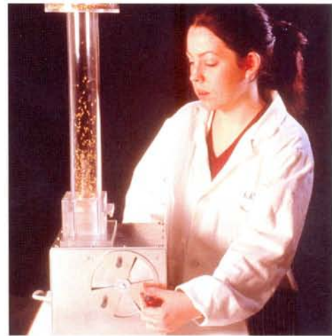
The quality of seed samples can be greatly improved by the use of an air column cleaner.
