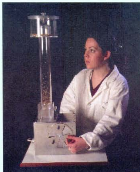
The quality of black-grass samples can be greatly increased by the use of an air column seed cleaner
