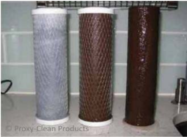
Figure 26. Build-up of iron deposits found on a water filter
