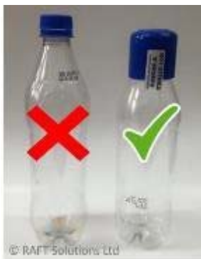
Figure 6. Example of a pre-sterilised water sample bottle suitable for microbiological analysis
