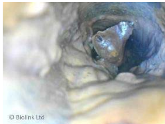
Figure 38. (left) Clean pipe and Figure 39. (right) Build-up of biofilm in a pipe
