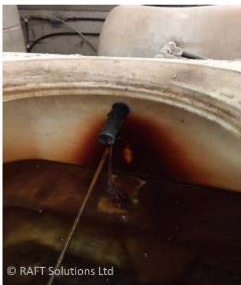
Figure 24. (left) and Figure 25. (right) Evidence of iron contamination found around the exit of a pipe and from the inside of a pipe
