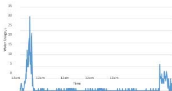
Figure 17. Example of backflow of water through a meter on a weaner site (Site 7)
