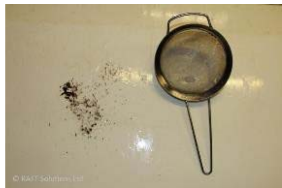
Figure 34. (left) and Figure 35. (right) Biofilm presence in a header tank
