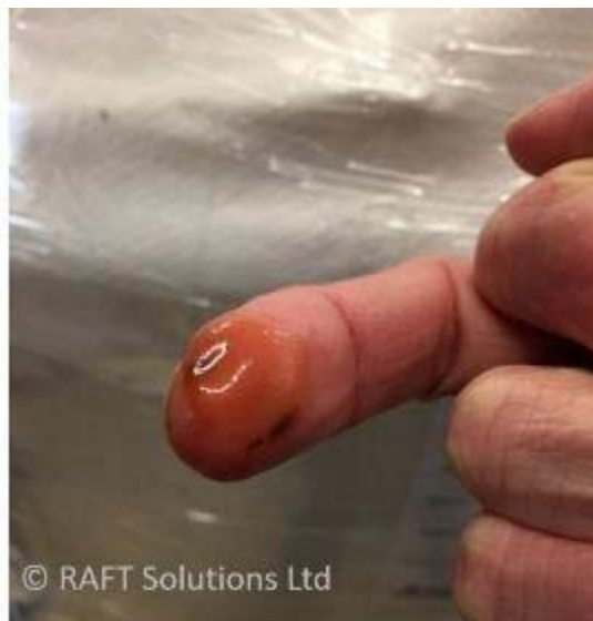
Figure 24. (left) and Figure 25. (right) Evidence of iron contamination found around the exit of a pipe and from the inside of a pipe
