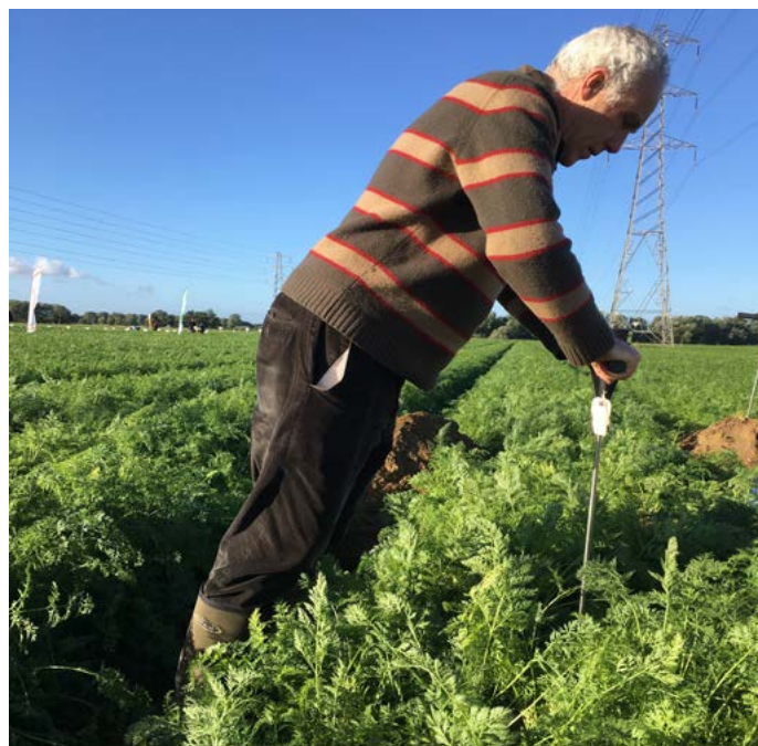
Figure 3. Martin Brittain (Fresh Growers) testing strength of soil in a carrot crop using a penetrometer
